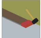
The end joints of this product features an integrated click-locking system with pushdown technology for an easy and speedy installation. Align the tongue and groove on the end joint of the next piece and press down. As the panel reaches is final position, the tongue flexes back
