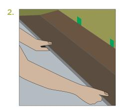
Position the first board in place by angling it up slightly, pushing forward and interlocking the side tongue. The long side of the plank or tile **MUST BE SNUG** against the adjoining plank or tile with **NO GAPPING.** If everything is aligned correctly, there will be a slight click from the end joint as the panel is successfully engaged and reaches its final position after being lowered into place.
