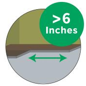
Maintain proper spacing (at least 6" for planks, and equal to half its length for tiles) between end joints for best appearance.
